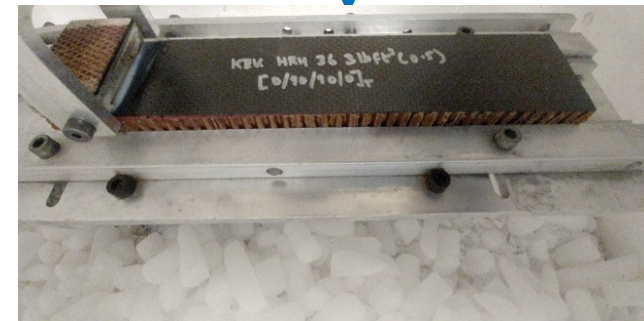
As-produced and environmental conditioned tested at -50°C
