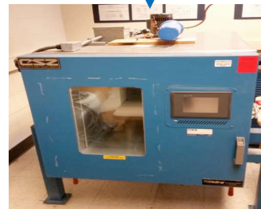
Witness panels exposed to humidity at 65°C and 90%RH
