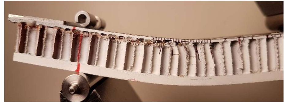
Core buckling in ENF test
