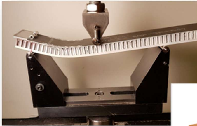
End Notch Flexure Test
