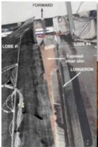
X-33 Liquid Hydrogen Tank Failure
