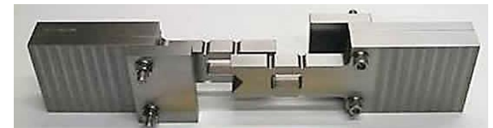
Open hole compression fixture for monolithic composites
