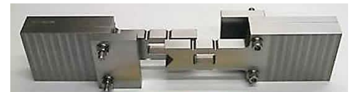
Open hole compression fixture for monolithic composites
