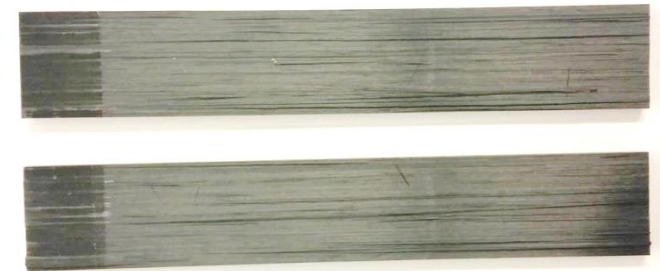
Composite Wedge Test Specimen
