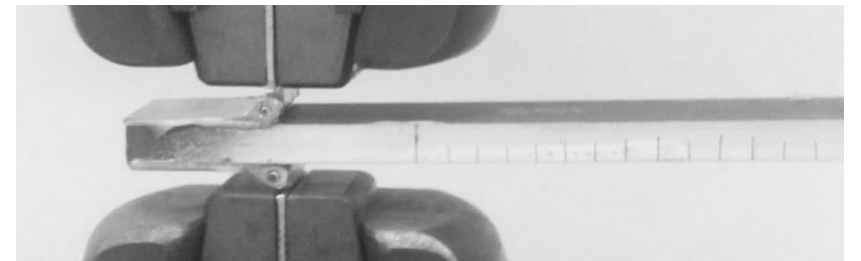
Double Cantilever Beam (DCB) Test
