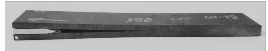
Composite Wedge Test
