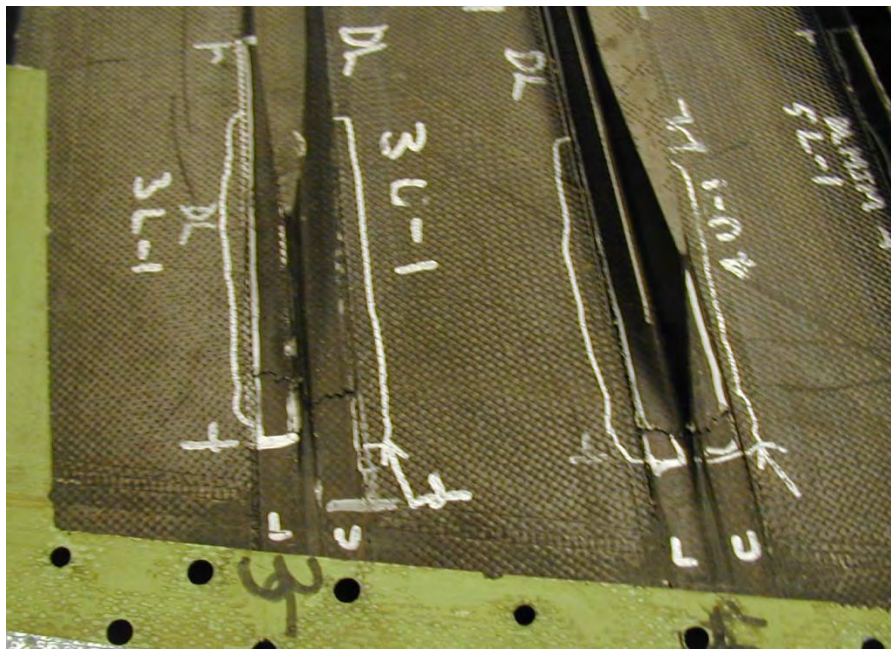
Upper skin Inboard delaminations at stringer runouts
