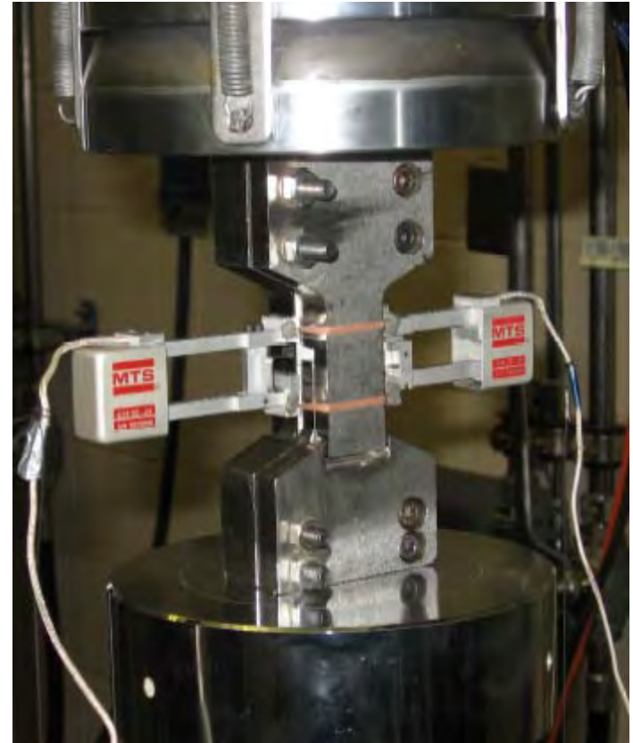
Compression Test Set-up
