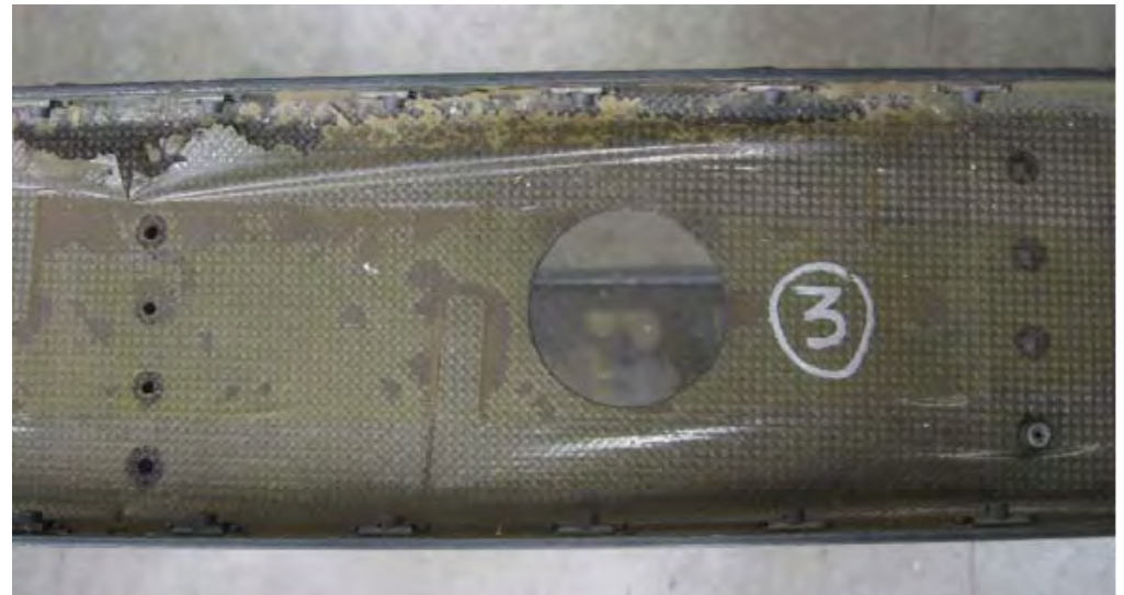
Degradation of Tedlar Moisture Barrier film
