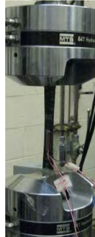
Tension Coupon Test Set-up
