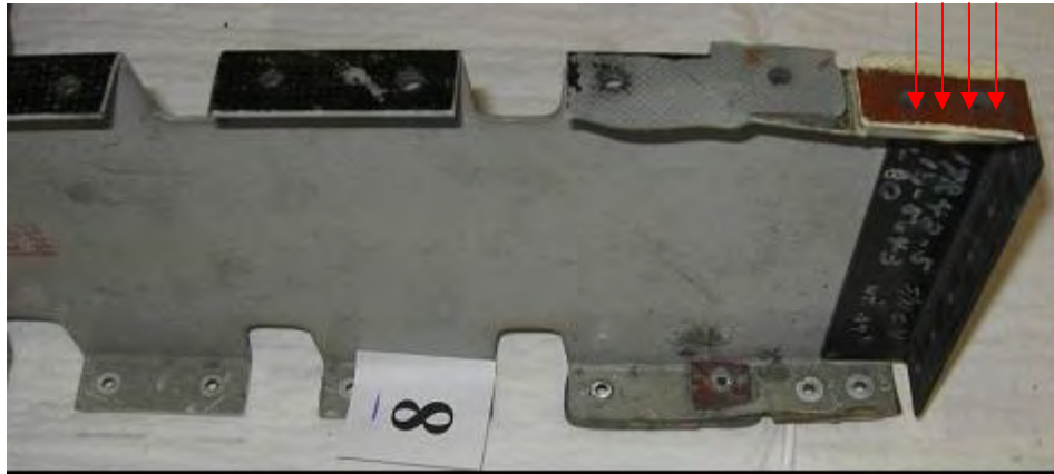
Phenolic shims used to fill gaps between skin and ribs
