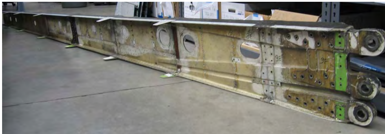
Front (Top) and Rear (Bottom) Spars after disassembly Wichita State University
