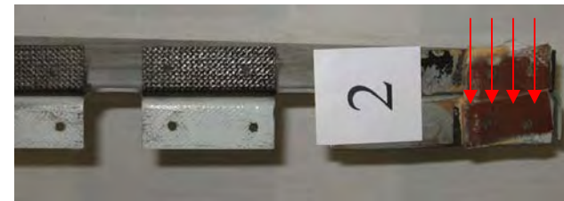
Phenolic shims used to fill gaps between skin and ribs
