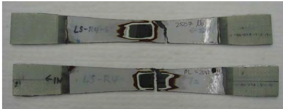
Tested Lower Skin Tension Coupons
