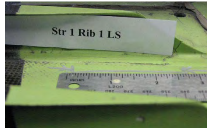
Upper skin Inboard delaminations at stringer runouts
