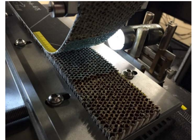
Disbond after Core Crush
