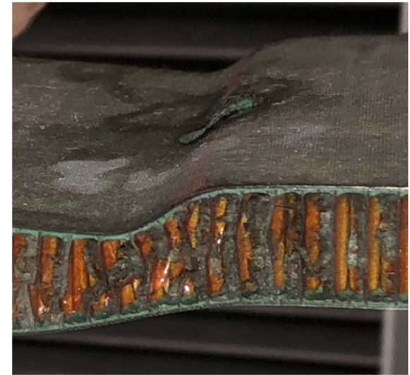
Sandwich Open-Hole Shear Failure
