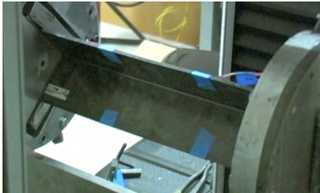
Specimen M3 at 3000 lbf ↔ 30,000 in-lbf
