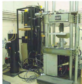
Piezoresistive type load cell PCB Model 206 M33 Platen Foot MTS hemispherical platen
