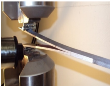
Adhesive Bond Strength Testing
