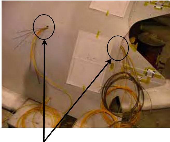
Wires routed through conduit in honeycomb core of inner sleeve.
