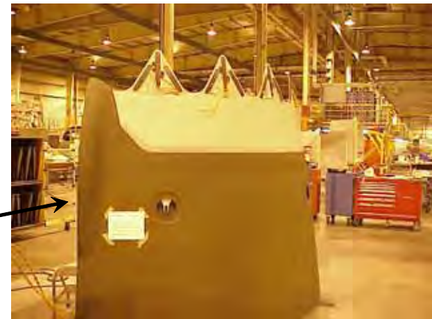
Outer Sleeve Joined to Inner Sleeve, wiring routed in space between sleeves
