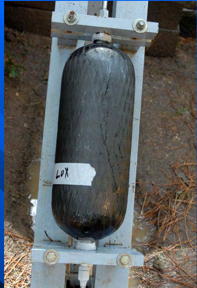
Over-wrapped, Aluminum Lined Pressure Vessels
