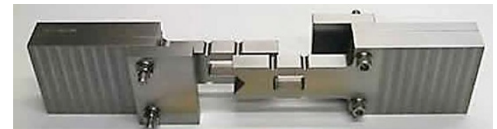
Open hole compression fixture for monolithic composites
