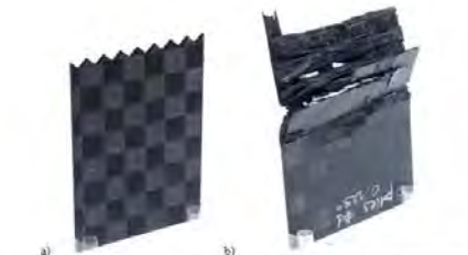
Figure 19 a, b Flat specimen, before crushing showing the saw-tooth trigger (a), and after crushing (b) at 12.5 mm of unsupported height
