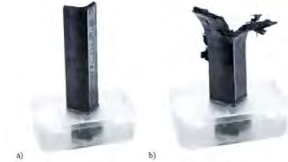
Figure 10 a, b. Small corner element, specimen IV, before and after crush testing
