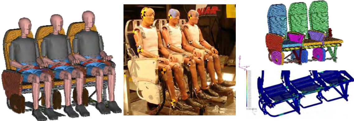
Figure 3. Strain Rate Domain Study for a Typical Part 25 Aircraft Seat Structure.
