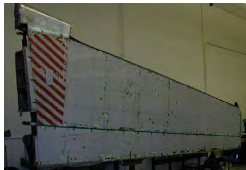
Figure (3). B-737 stabilizer configuration. Figure (4). B-737 composite stabilizer after 18 years of service.
