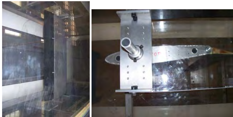
Figures: Fin / rudder aeroelastic wind tunnel model (composite rudder allowing for testing the effects of hinge failure)
