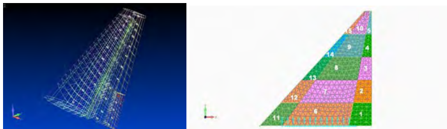
Figures: Passenger airplane fin / rudder NASTRAN model and simple prototype plate-like wing NASTRAN wing model for aeroelastic reliability studies
