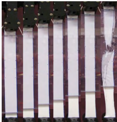
Figure 3: Stretching Behavior of Membrane and Ultimate Failure
