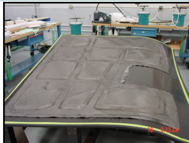
Dry Fiber lay up Process
