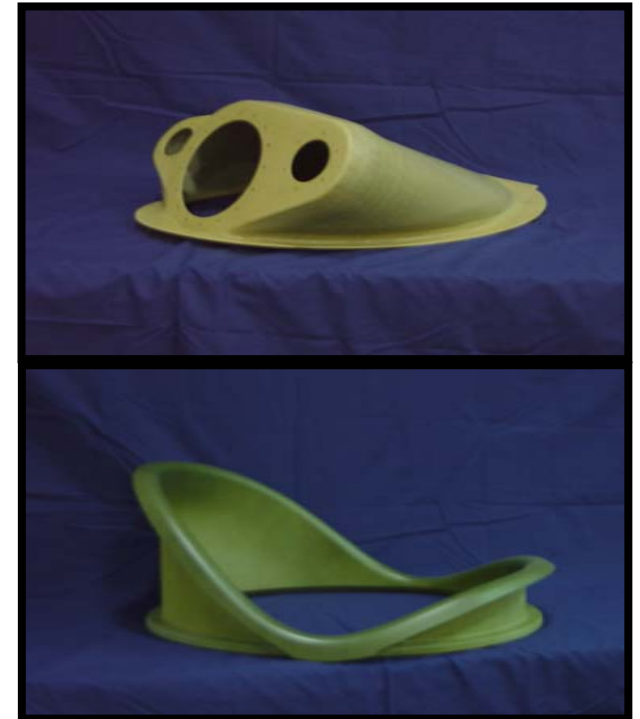
757 APU Inlet Ducts
