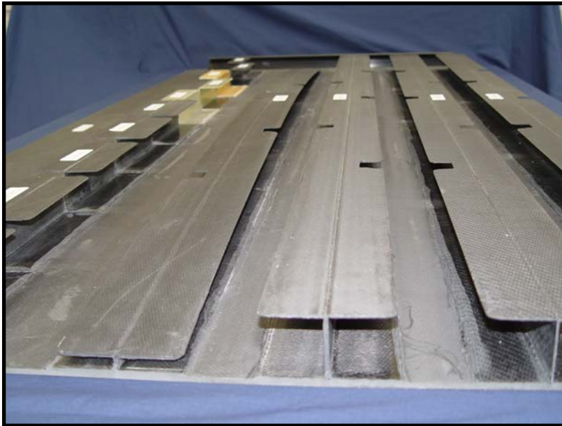
VARTM Infused Panel With Integral Stringers
