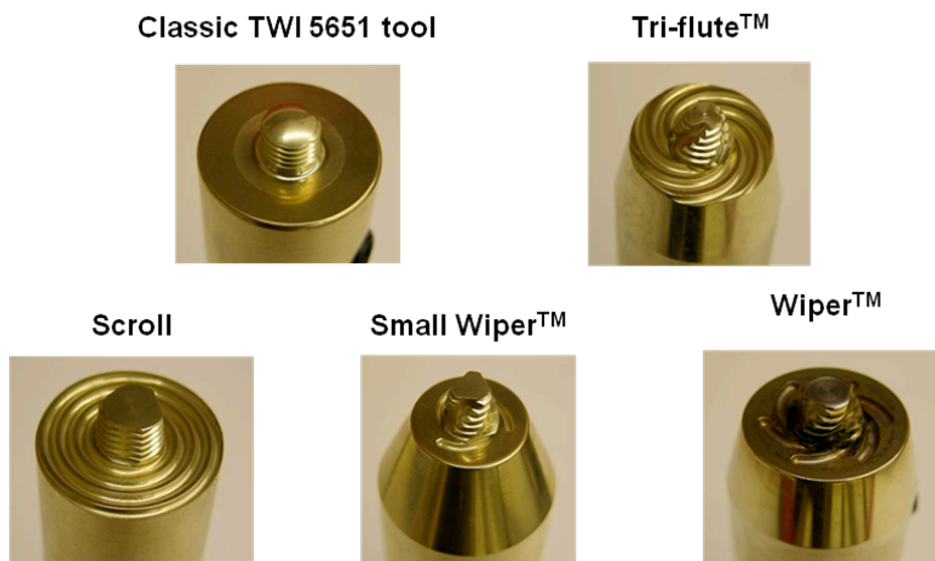
Figure 3. Tool designs include the classic TWI 5651, Tri-flute™, Scrolled shoulder with threaded pin and straight flats, Small (shoulder) Wiper™ with threaded pin and twisted flats, and a Wiper™ (large diameter shoulder) with threaded pin and twisted flats. 1,12
