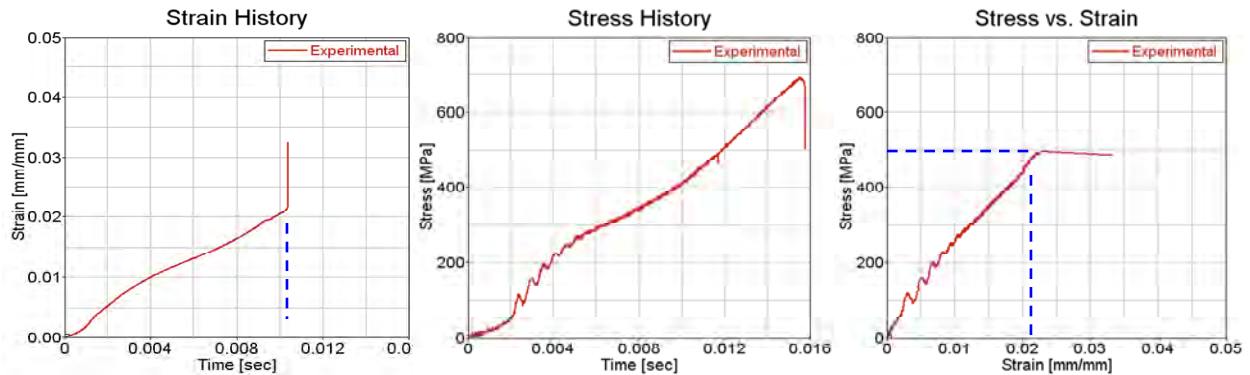
Figure 19. Stress-strain curve limited by strain gage capability.
