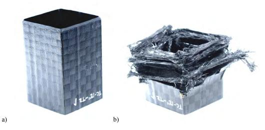
Figure 4. Square tube, specimen I, before (a) and after crush testing (b).
