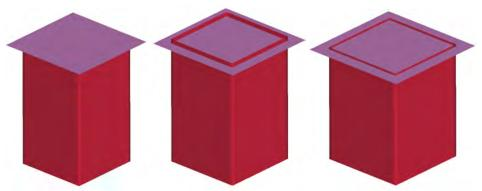
Figure 14. Example of a stable crushing of the tubular shape with SOFT=0.08. No buckling.
