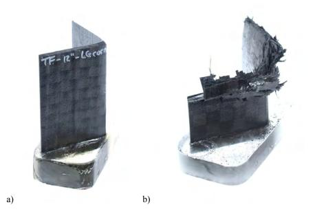
Figure 8. Large corner element, specimen V, before (a) and after crush testing (b).
