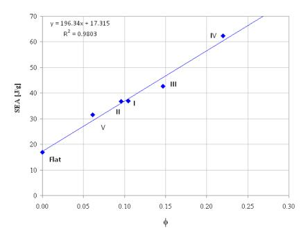
Figure 10. SEA variation with  $\phi$ , which is an indicator of curvature per unit length of cross-section for all specimens tested.
