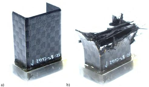
b) Figure 5. Large C-channel, specimen II, before (a) and after crush testing (b).
