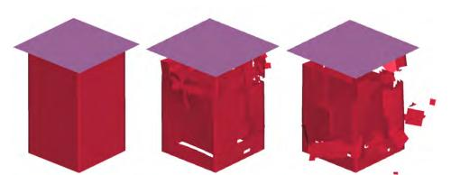
Figure 12. Example of an unstable crushing of the tubular shape with SOFT=0.64 Buckling starts after 2.446 millsec at a displacement of 0.3669 inches.
