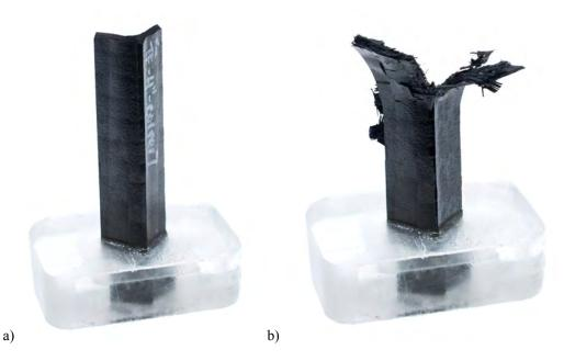
Figure 7. Small corner element, specimen IV, before (a) and after crush testing (b).
