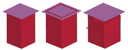
Figure 13. Example of an unstable crushing of the tubular shape with SOFT=0.3. Buckling starts after 3.728 millsec at a displacement of 0.5592 inches.
