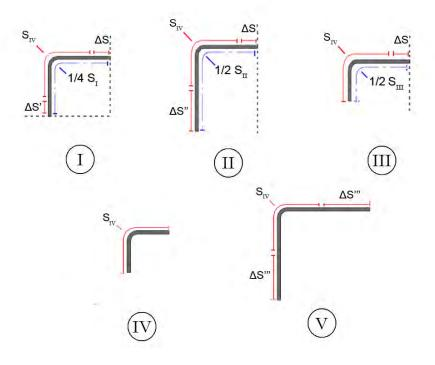
6 American Institute of Aeronautics and Astronautics Figure 4. Subdivision of section length into a corner detail and portion of flat segments, for each of the five specimen cross-section geometries considered.
