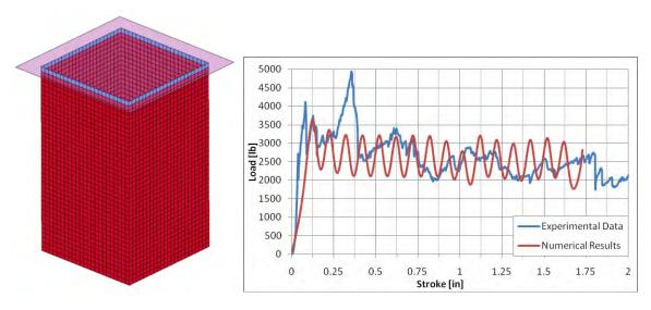
Figure 16. Model geometry and optimal Load-Displacement curve for the square tube specimen
