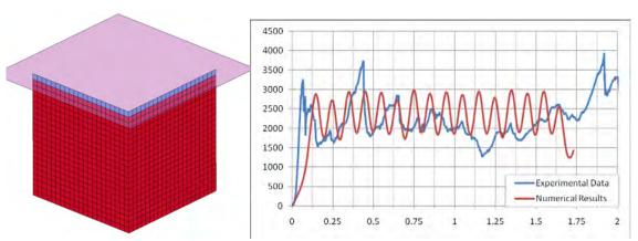
Figure 20. Model geometry and optimal Load-Displacement curve for the large Corner specimen
