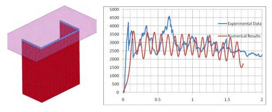
Figure 17. Model geometry and optimal Load-Displacement curve for the large C-Channel specimen.
