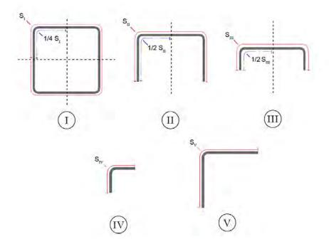
Figure 2. Illustration of the concept of section length for each geometry considered, and portion of such length influenced by a single corner detail.
