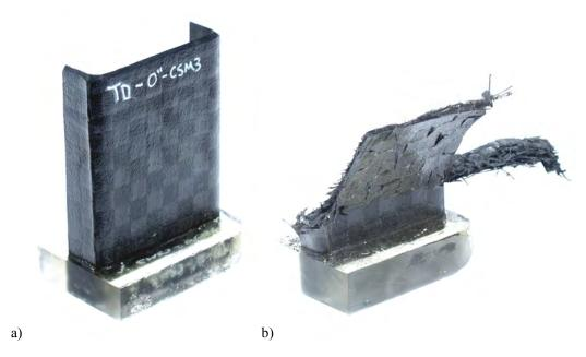
Figure 6. Small C-channel, specimen III, before (a) and after crush testing (b).
