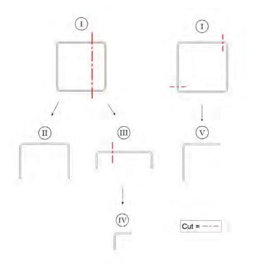
Figure 3. Shematic of machining operation performed to obtain test specimens II through V beginning from specimen I.
