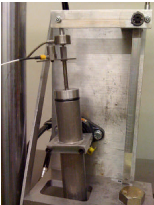
Figure 14: The damper in the Instron machine: Lever attachment arrangement
